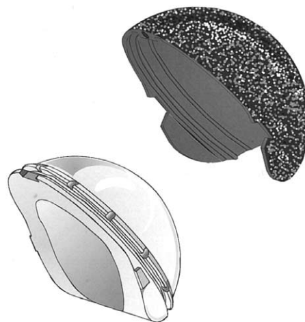
Fig. 1. The Buechel-Pappas Acetabular Component with the anatomic design and inferior cutout.
